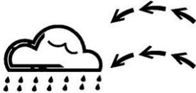
The storm threshold can be set to suit the user's requirements for storm forecasting - anywhere from 3-9hPa (default 4hPa). When there is a fall below the pressure threshold within any given 3 hour period the clouds with rain icon as well as the tendency arrows will flash for 3 hours indicating the storm warning feature has been activated.
