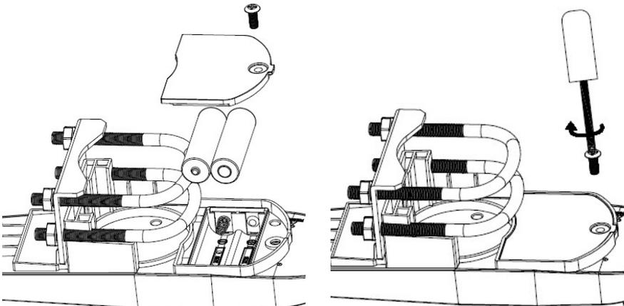
**Figure 7: Battery installation diagram**
