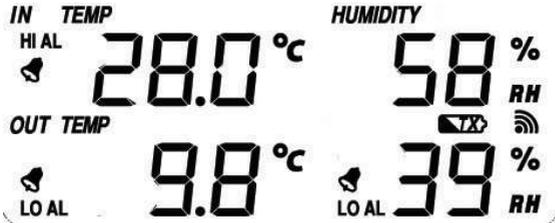
Press the **MENU** key eight times to select the INDOOR TEMPERATURE section, the INDOOR TEMPERATURE section digits will start flashing. Press the **UP** or **DOWN** key to change the temperature unit between °C and °F.
