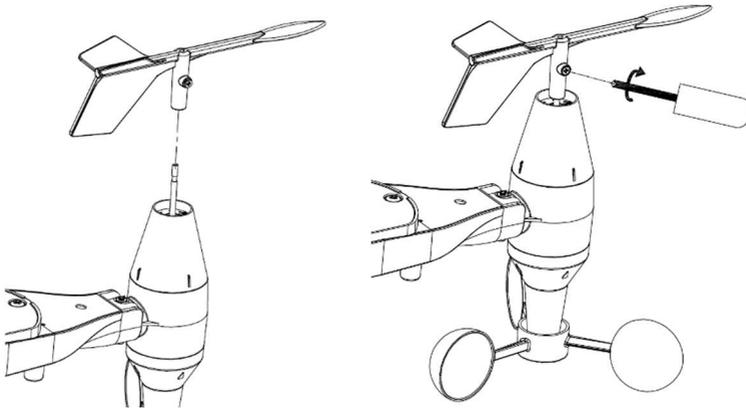
**Figure 6: Wind vane installation diagram**
