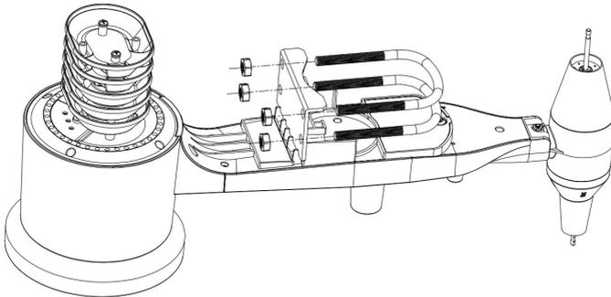
**Figure 3: U-Bolt installation**
