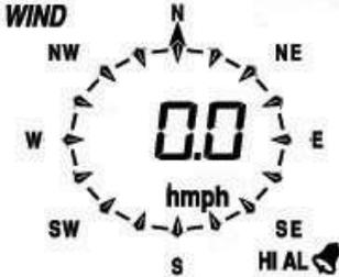
Press the **MENU** key three times to select the WIND section, the WIND section digits will start flashing. Press the **UP** or **DOWN** key to shift the display between Average wind speed and Gust (default Average wind speed).
