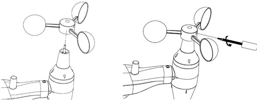
**Figure 5: Anemometer installation diagram**
